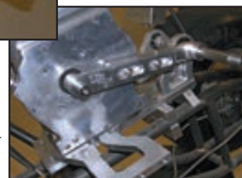
Using clutch tool to set center to center distance.
